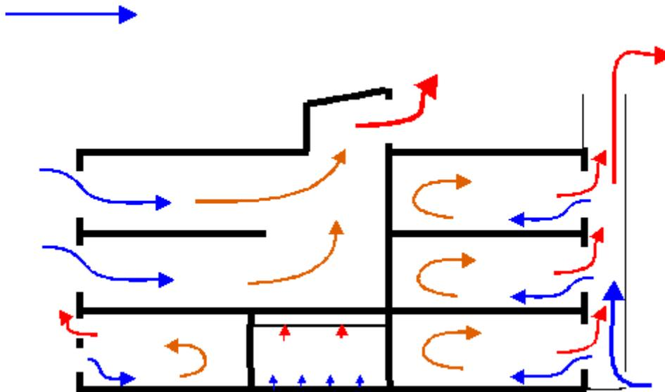
Any combination of ventilation regimes can be included in the same building model. Control of open area for windows etc can be placed under the influence of a range of internal variables and in addition linked to climate parameters. Aperture opening can be controlled individually or in groups from the performance of any space or group of spaces. Solar control devices may also be operated with the same level of flexibility in combination with the modulation of openings.
