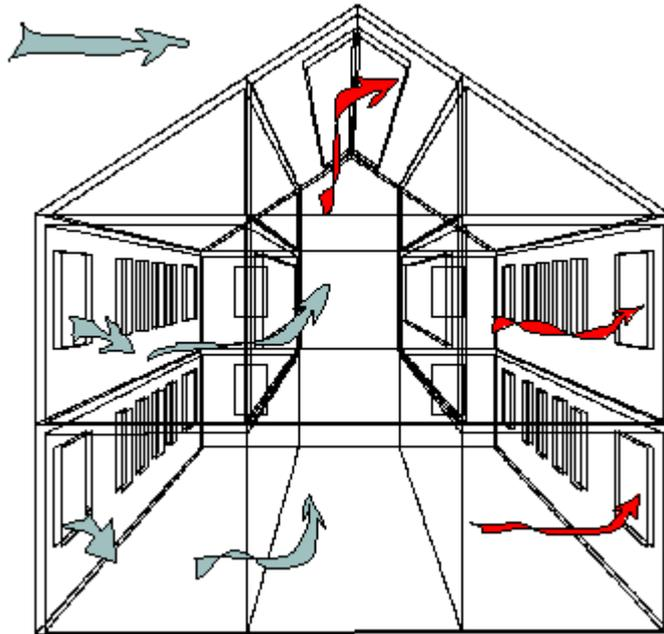
Using recorded hourly weather data containing solar radiation, air temperature and wind speed and direction, an energy and air flow balance is calculated at hourly time steps. Simple cross ventilation is evaluated on wind speed and direction, modified by the relative height of openings and surrounding buildings. Single sided ventilation is based on the internal to external temperature difference and the physical height of the openings.
